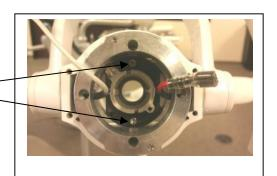
Apply pressure to the open end of the socket and push it through the back of the bushing assembly.
