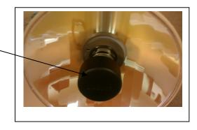
4. Remove light reflector. Turn the light reflector counter clockwise to loosen it. Once loose continue to turn the retaining nut to remove the reflector.
