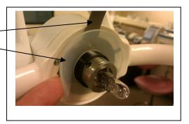
Disconnect the light bulb and common power line wire from the socket. Brass Phillips screw.
