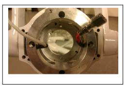
10. Replace the light socket and reverse the above steps to complete. Make note of the orientation of the light socket. Be sure to install the socket with the adjustment screw in the correct position. This screw will protrude through the light handle so that adjustments can be made.
