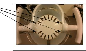
2. Remove the Phillips head screw that attaches the shield.
